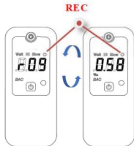
In the record mode, the test number and its reading will flash on the LED alternatively. For example, the 9<sup>th</sup> record is **0.58‰ BAC (= .058% BAC)**, then r09 and 0.58‰ will flash alternatively.
