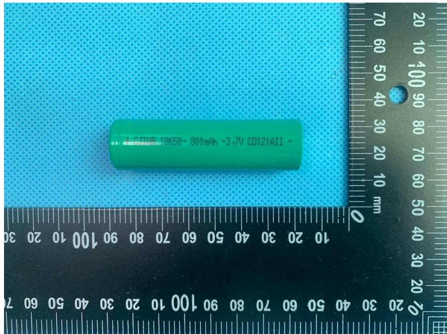
Figure 1 Front view of cell (Model: INR 18650-800mAh)
