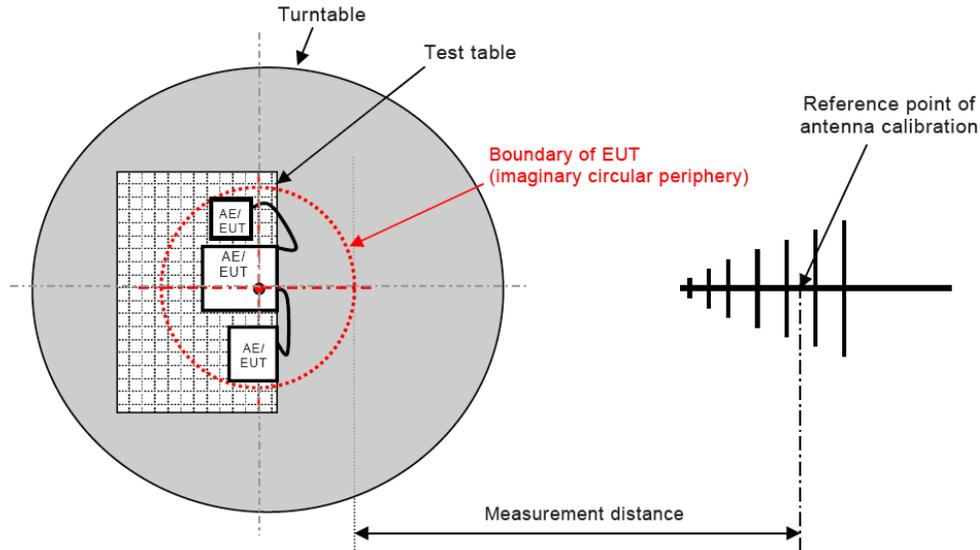
The radiated emission tests were performed in the open area 3-meter test site, using the setup accordance with the CISPR 16-1-1: 2019, CISPR 16-2-3: 2010. The specification used was EN 55014-1: 2020
