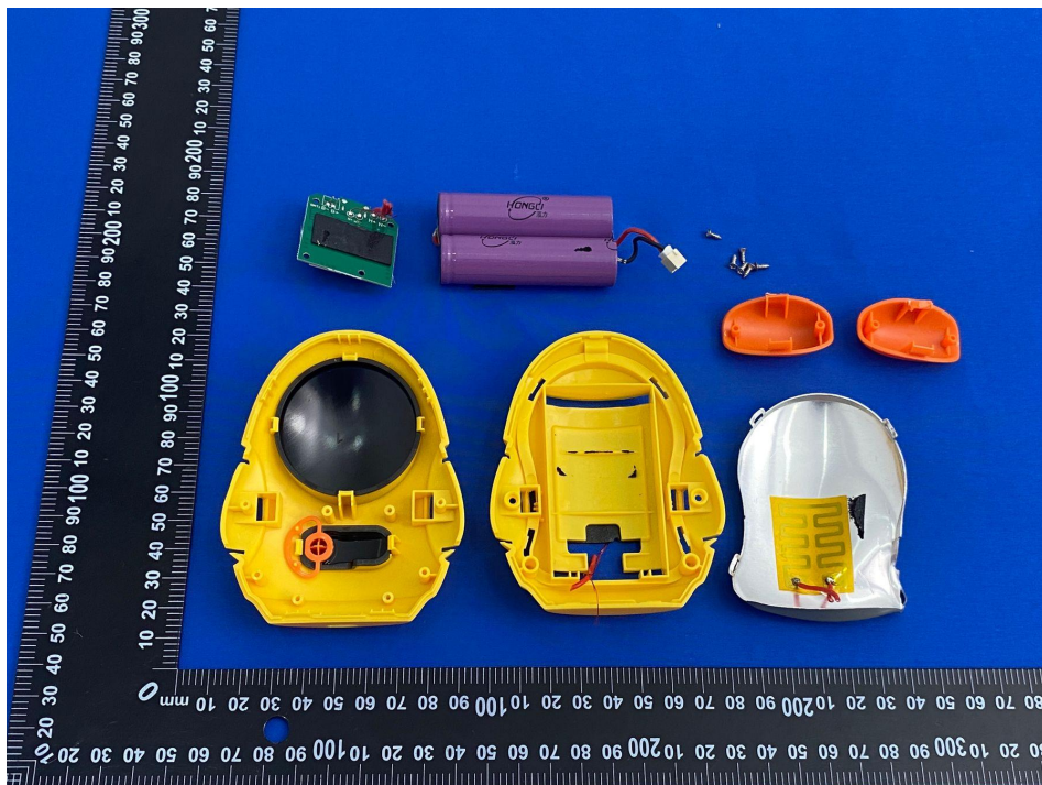
Photo 4 Inside of EUT
